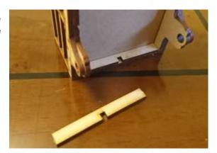
Insert the centre cross beams into the slots in the sole bars, again with the central slot faving away from the wagon floor
