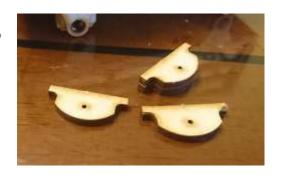
The final task is to glue the top flange onto the wagon
