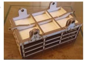
Glue the bearings into the axleboxes from the inside ensuring that the flange is completely flat to the inner sole bars. Be very careful not to allow glue to enter the bearing Then, before the glue is dry, insert the Axle rod through the axleboxes as shown
