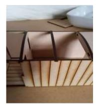
Chamfer the top edge of the guards van sides so they match the contour of the roof supports.
