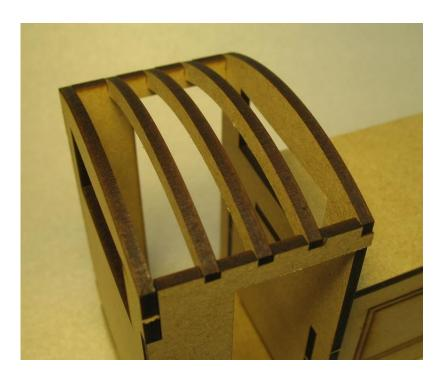
Be generous with the glue when attaching the roof. Hold it in position with strong rubber bands until the glue has set.
