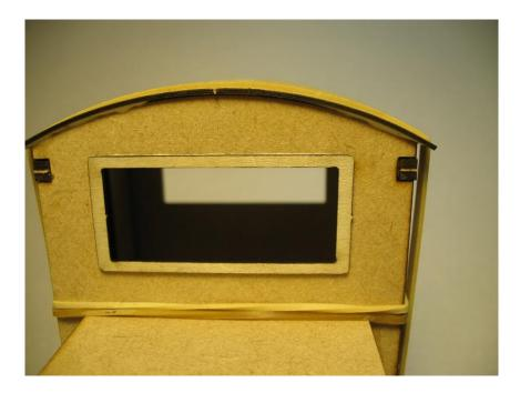
Glue the aluminium mesh onto the supplied frame. Epoxy is the best glue for this. Once the glue is set trim off the excess mesh. Mount it inside the engine cover once the loco has been painted.
