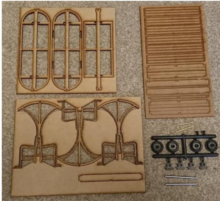
Start by carefully separating the parts from their sheets. Wiggling them lightly is normally enough to break the retaining tab. Sand or file the retaining tabs away on all parts before beginning assembly.
