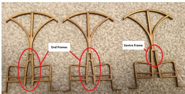
Identify the difference between the upright frames. The two end frames have a rectangular hole for the backrest and two locating lugs at the bottom. The centre frame has no locating lugs and a slot for the backrest.
