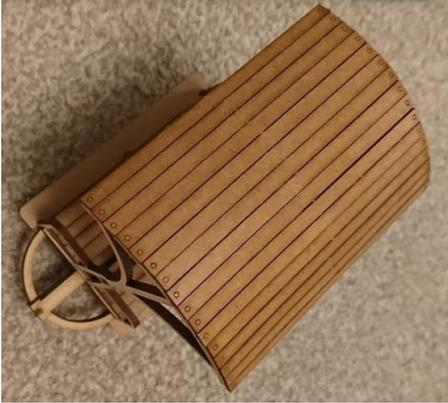
Glue on the planks of the parasol roof with the coach bolt detail uppermost. There are 16 planks for the roof, (plus a couple of spares because these delicate parts are easily damaged until glued in place on the Sitzwagen)
