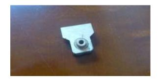
Before gluing the axle boxes onto the chassis do a dry fit by placing one or two washers between the wheel set and bearing to ascertain how tight you want the axles to be in the frame. One washer on each side gives a fair amount of sideways play to allow for less than perfect track, two allows less sideways play.
