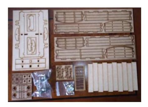
If not already done start by carefully separating the parts from their sheets. Wriggling them lightly is normally enough to break the retaining tab. Sand the retaining tabs away on all parts before beginning assembly.
