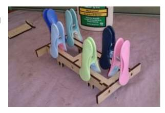
Glue the two halves of each buffer together
