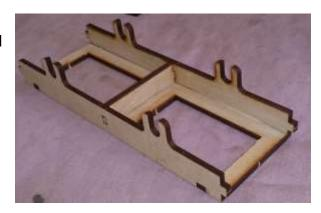
Glue the buffer beams onto the sub frame. Either elastic bands or domestic clothes pegs can be used for clamping while the glue sets.
