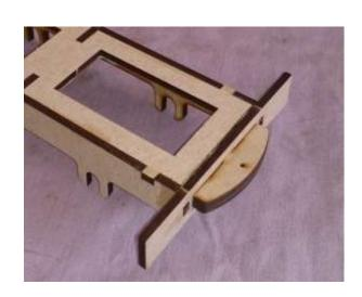
Assemble the axle boxes by layering the three parts for each axle box. Inner mounting (with large hole), then spacer (with small hole) finally outer end cap
